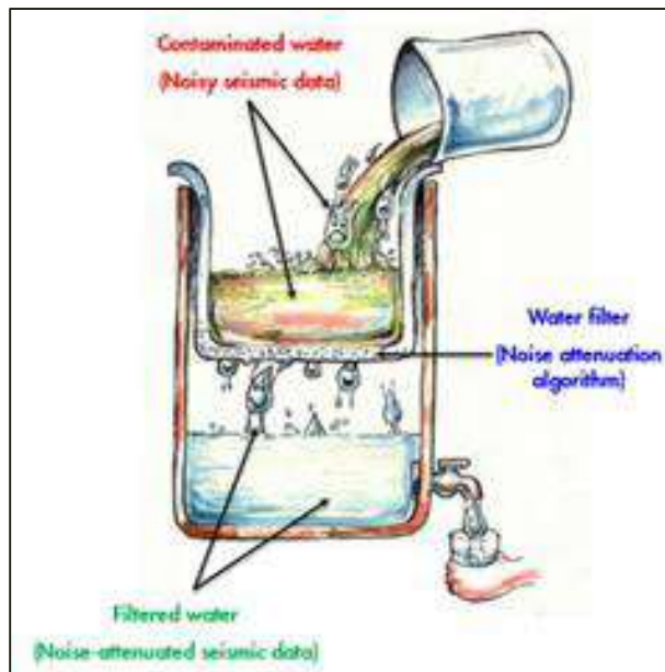
Figure 3: A schematic to illustrate the concept of Noise attenuation likened like a water filter purifier.
