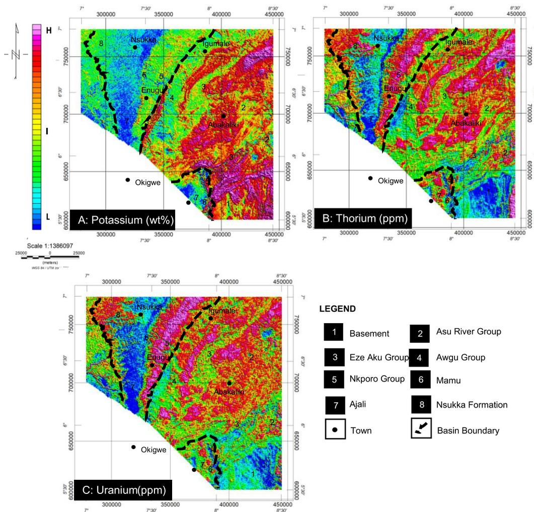
**Figure 3:** Radiometric maps used (A) Potassium (B) Thorium (C) Uranium concentration maps.
