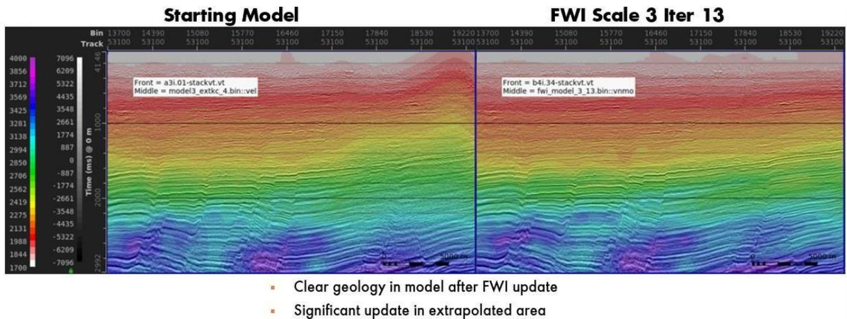
Figure 8: Inverted velocity model overlain on the seismic data Comparing the old PSDM model (top left) and the new PSDM model (top right) clearly shows the amount of detail that has been brought into the velocity model using the techniques described in this paper. The validation of the details is done by co-rendering the new PSDM model with the seismic (bottom). The variations in the velocity model are clearly consistent with the fault blocks.
