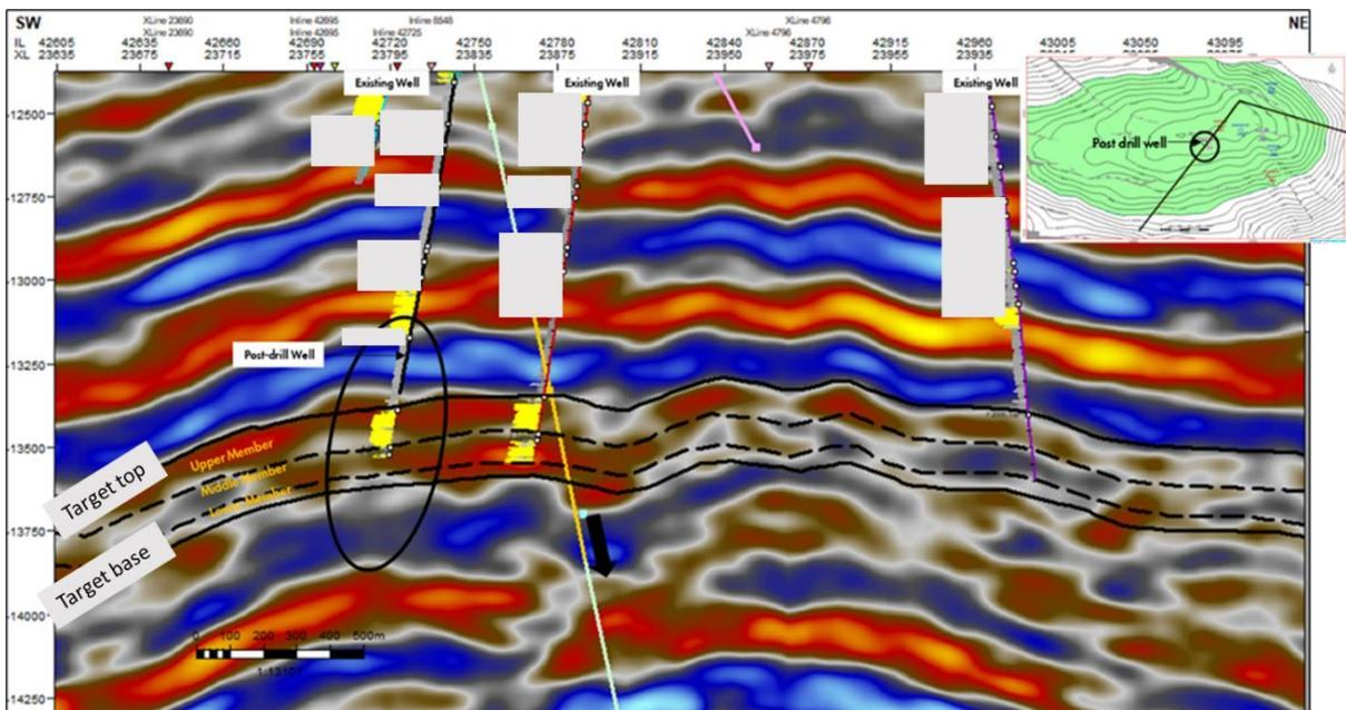
*Figure 15: Post drill seismic relative impedance section across the target reservoir. Thickness and property prediction encountered is with pre- drill range of prediction.*
