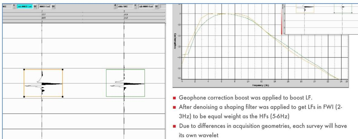
Figure 4: Wavelets for Survey A and Survey B
