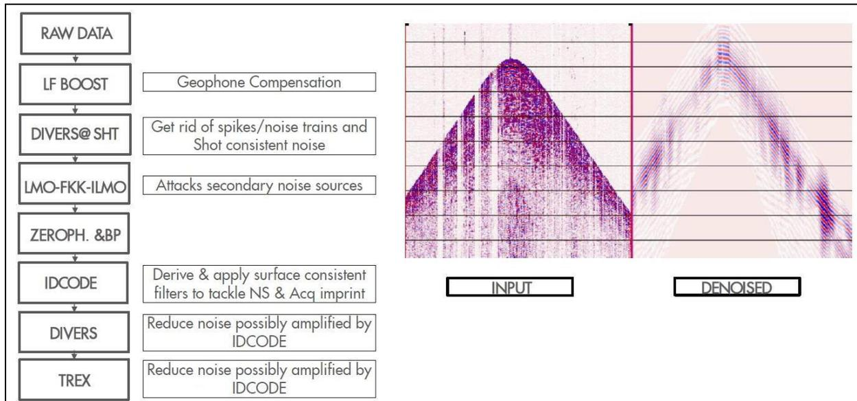
Figure 5: Pre-processing workflow applied with the results
