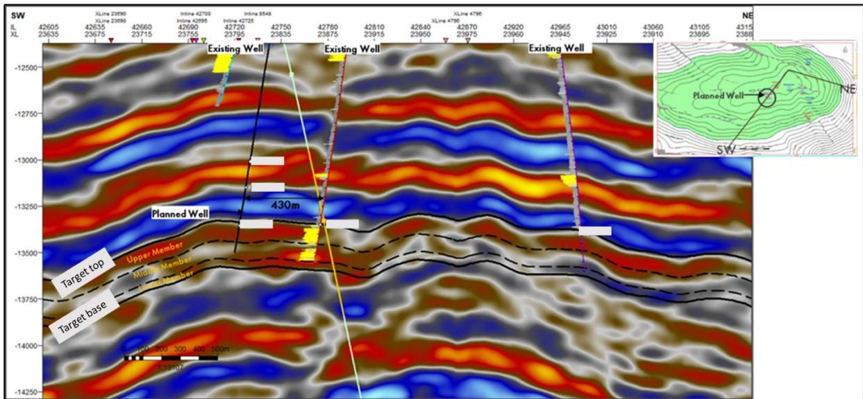
Figure 14: Relative Impedance Section Cross the planned well showing the expected stratigraphy of the F2000 reservoir along the planned well path.
