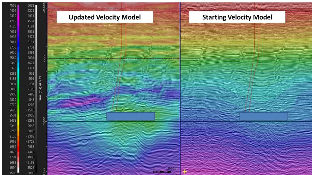
Figure 11: FWI + Sonic velocity model. The details from the velocity model are geologic and conforms to structural and stratigraphic changes.
