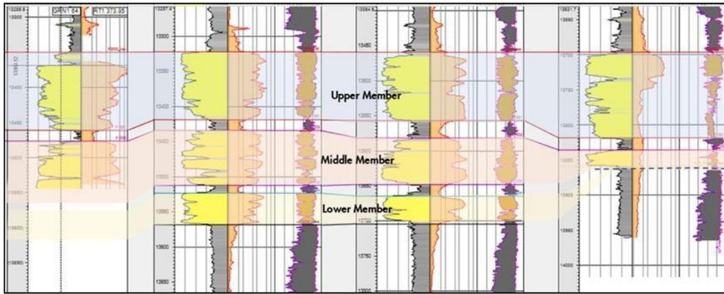
Figure 13: Stratigraphic correlation across the existing wells in the target reservoir showing the three sand members of the reservoir)
