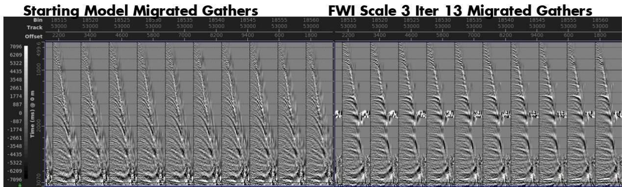
Figure 7: Migrated gathers showing improved quality of the velocity model after scale 3 iteration 13
