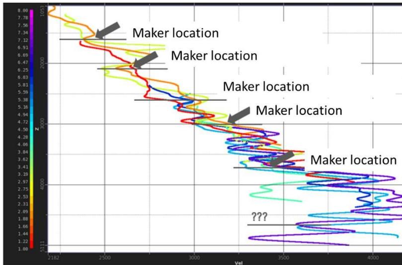
Figure 9: Plot of selected sonic logs in study area with proposed geological markers
