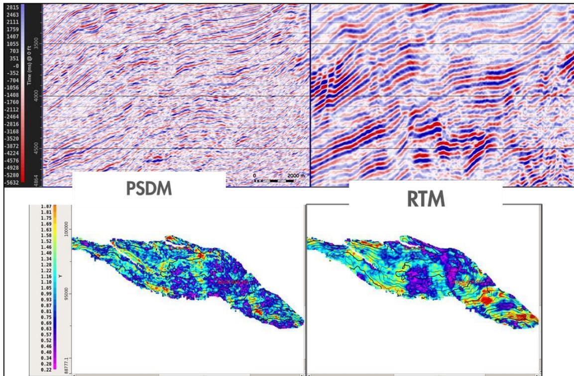
Figure 12: Comparing the old PSDM model (top left) and the new PSDM model (top right). Amplitude extraction of legacy (bottom left) and new seismic (bottom right)
