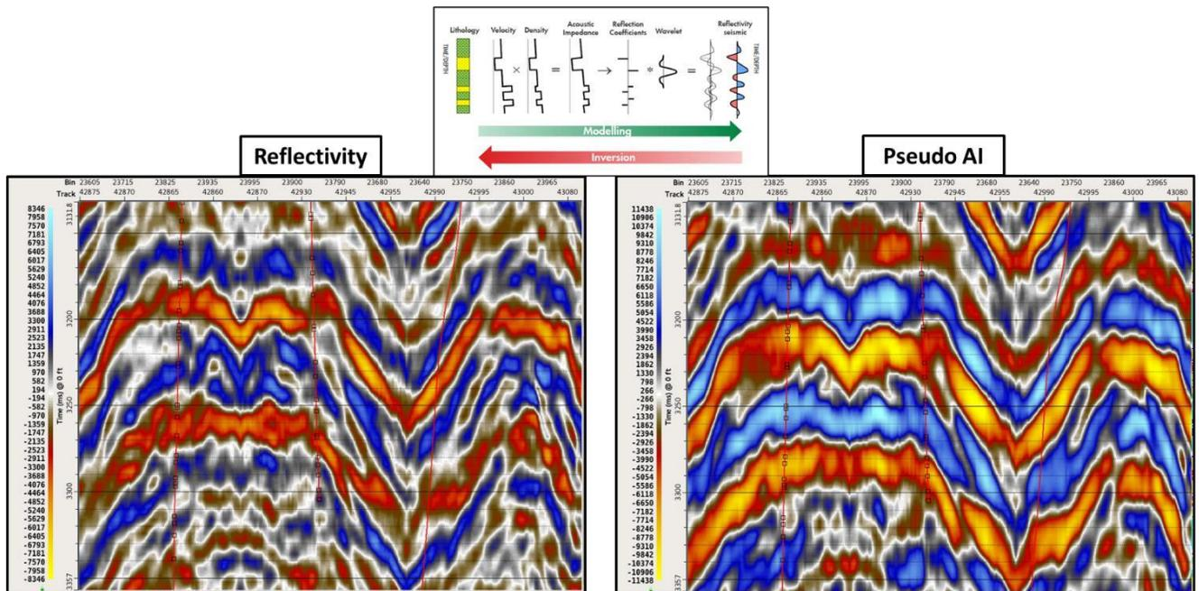
Figure 14: comparison of the reflectivity seismic volume and the relative acoustic impedance seismic volume: the reflectivity showed the rock interfaces while the relative AI showed the rock layers and are smoother.
